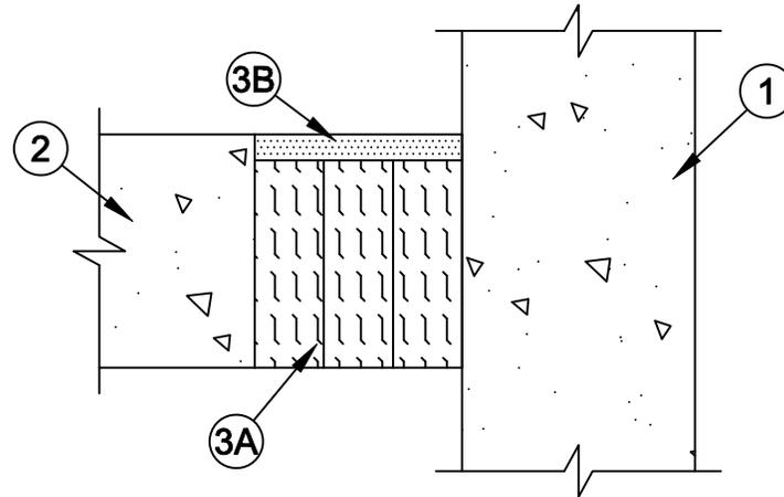
1. **Wall Assembly** - Min 4-1/2 in. (114 mm) thick reinforced lightweight or normal weight (100-150 pcf or 1600-2400 kg/m3) structural concrete. Wall may also be constructed of any UL Classified **Concrete Blocks\***. See **Concrete Blocks** (CAZT) category in the Fire Resistance Directory for names of manufacturers.
