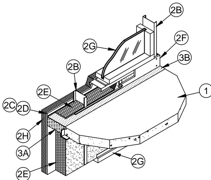
1. **Floor Assembly** - Min 4-1/2 in. (114 mm) thick reinforced lightweight or normal weight (100-150 pcf or 1600-2400 kg/m<sup>3</sup>) structural concrete. Perimeter of floor assembly to be provided with min 3 by 3 by 1/4 in. (76 by 76 by 6 mm) thick cast-in-place structural steel angle for weld-attachment of mounting angles (Item 2A).
